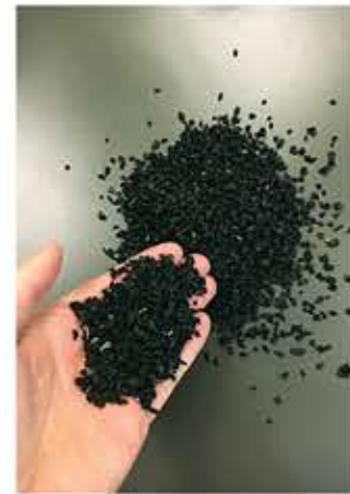
Output: 16 - 4 mm (0.625" - 0.16" -inch) and smaller crumb rubber
