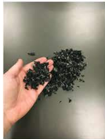
Output: 38 - 16 mm (1.50" - 0.625"-inch) and wire-free rubber mulch/chips.
