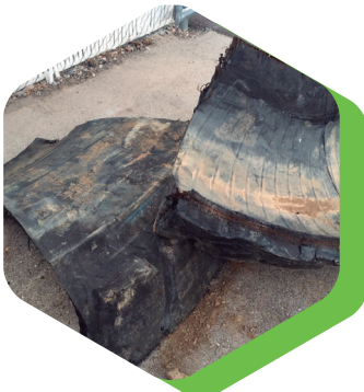
Sheared chunks after being split by the Eco Razor
