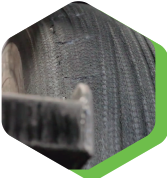
Removal of high quality rubber from tread and side walls
